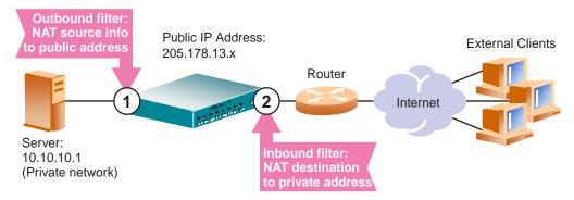
Figure 7-8 Static Network Address Translation
